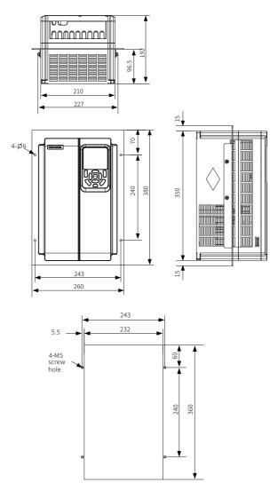
Figure 1-13 Dimensions of MD500-AZJ-A1T5 through-hole mounting bracket and holes (mm)
