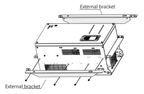
The following figure shows an AC drive with brackets mounted.
