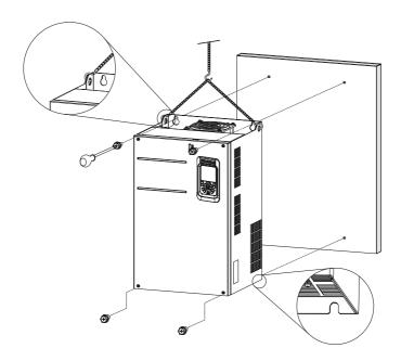
Figure 4-9 Backplate mounting (T7 to T9 models)
