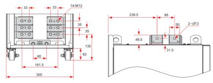
Figure 7-18 Main circuit terminal dimensions of T10 models (without side copper busbars and output reactors) (mm)
