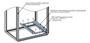
Figure 5-7 Installing the bottom mounting bracket
