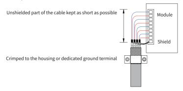
Figure 7-51 Handling shielded cables
