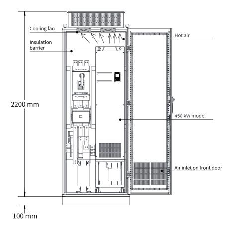
Figure 5-2 Force-ventilated cabinet (with top-mounted fans)
