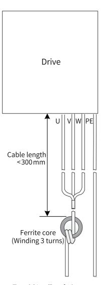
Figure 8-2 Installing a ferrite core
