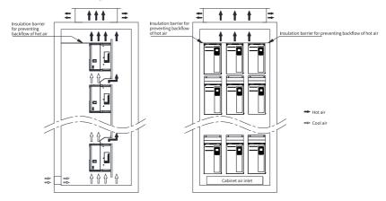
Figure 4-5 Backflow of hot air in a self-ventilated cabinet (with an insulating device)
