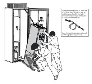
Figure 5-11 Pushing the AC drive into the cabinet
