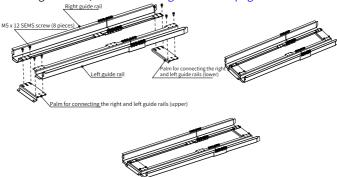
Figure 5-8 Assembling guide rails
