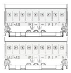
Figure 7-3 Main circuit terminals of T2 models (single phase)
