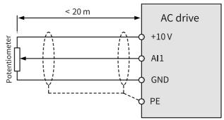
Figure 7-32 Wiring analog input terminal AI1
