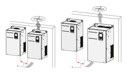
Figure 1-4 Installing multiple AC drives (T1 to T9 models) side by side  $\,$
