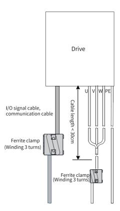
Figure 8-3 Installing a ferrite clamp
