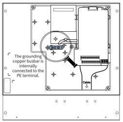
Figure 7-44 PG card installation screws
