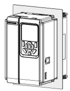
2. Fasten the AC drive with the bracket onto the mounting backplate of the control cabinet.
