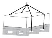
Figure 3-1 Hoisting the AC drive
