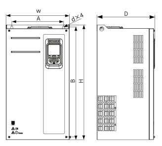
Figure 2-3 Outline dimensions and mounting dimensions of T7 to T9 models
