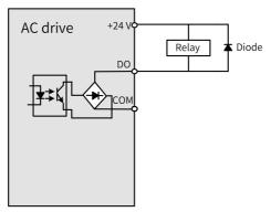
Figure 7-38 Wiring a DO terminal
