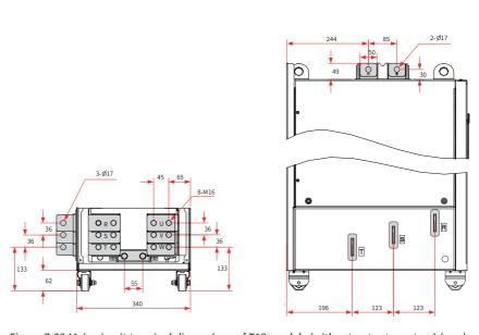
Figure 7-22 Main circuit terminal dimensions of T12 models (without output reactors) (mm)
