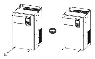
b. Hold the cover with both hands, and pull it in the arrow direction to remove it.
