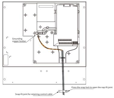
Figure 7-43 Grounding the shield of analog input cable
