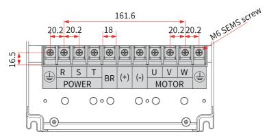
Figure 7-12 Main circuit terminal dimensions of T6 models (mm)
