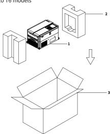
Figure 3-3 Packing list for T1 to T6 models
