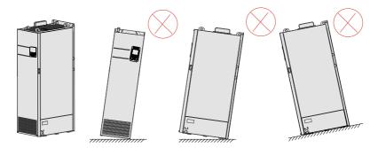
Figure 1-8 Installation direction (T10 to T12 models)
