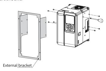
The following figure shows an AC drive with a bracket mounted.
