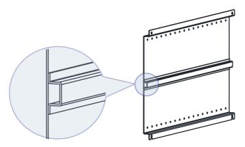
Figure 4-2 Welding a lateral reinforcing beam on the back of the backplate
