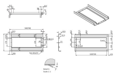
Figure 1-19 Dimensions of bottom mounting bracket for T11 models
