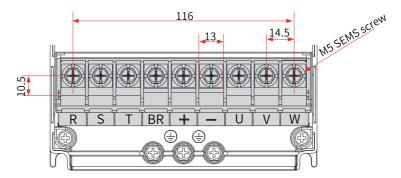
Figure 7-9 Main circuit terminal dimensions of T3 models (mm)
