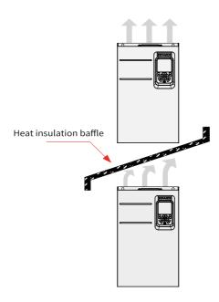
Figure 1-5 Installing one above another
