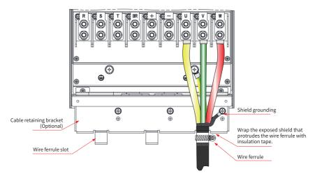
Figure 4-11 Wiring of the cable shield
