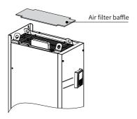
Figure 5-13 Removing the air filter baffle
