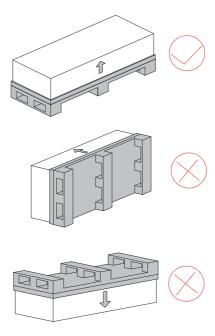
Figure 3-2 Placing the AC drive
