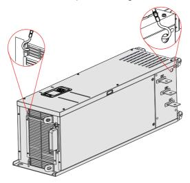
Figure 3-9 Hoisting T10 to T12 models
