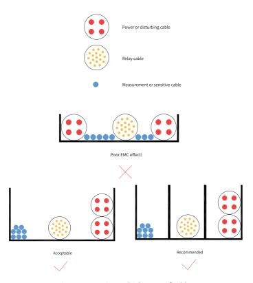
Figure 7-50 Laying multiple types of cables
