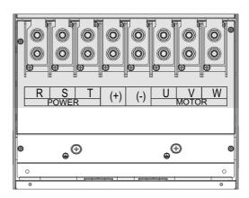
Figure 7-6 Main circuit terminals of T9 models
