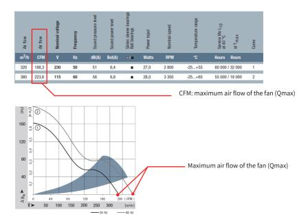
Figure 4-6 Q max of a system fan
