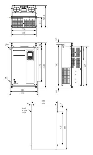
Figure 1-16 Dimensions of MD500-AZJ-A1T8 through-hole mounting bracket and holes (mm)
