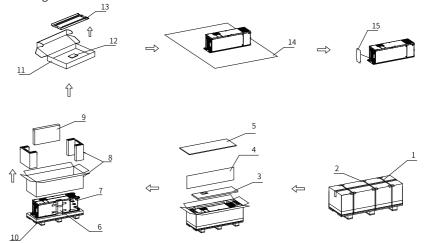
Figure 3-5 Packing list for T10 model
