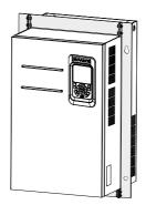
2. Fasten the AC drive onto the backplate of the control cabinet from the front of the control cabinet.
