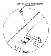
Figure 9-1 Disconnecting the optional EMC grounding screw
