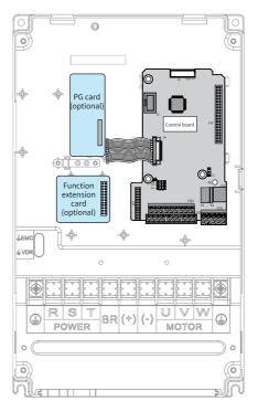
Figure 4-10 Position of the control board
