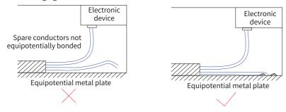
Figure 7-48 Handling reserved core wires of multi-conductor cables
