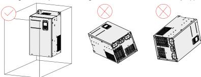
Figure 1-7 Installation direction (T1 to T9 models)
