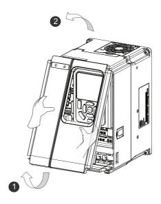
The following figure shows an AC drive with its cover removed.
