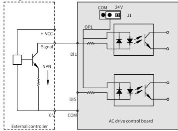
Sink wiring where the 24 V power supply of the AC drive is used
