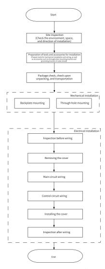
Figure 1-1 General installation process (T1 to T9 models)
