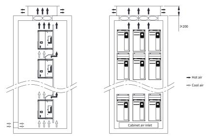
Figure 4-7 Cabinet ventilation system
