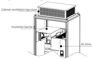
Figure 5-3 Insulation barrier in the cabinet
