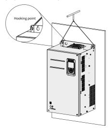
Figure 3-8 Hoisting T1 to T9 models
