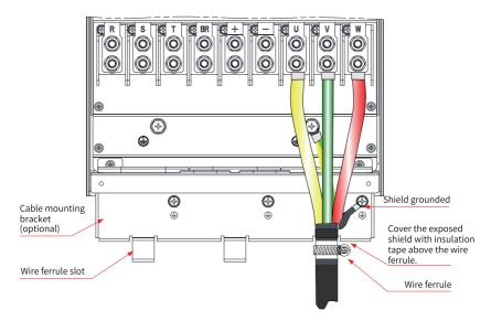
Figure 7-28 Shield wiring
