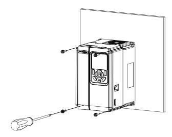
Figure 4-8 Backplate mounting (T1 to T6 models)
