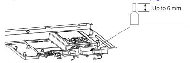
Figure 7-40 Requirements on the tubular terminal of a control cable
