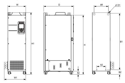
Figure 2-4 Outline dimensions and mounting dimensions of T10 to T12 models (without AC output reactor)
