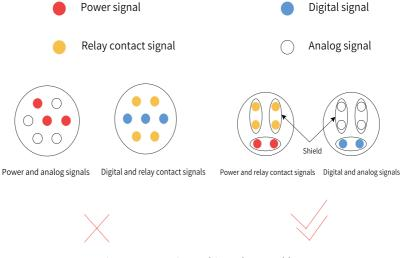
Figure 7-47 Routing multi-conductor cables
