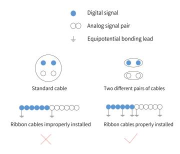
Figure 7-46 Routing cables that transmit different types of signals
