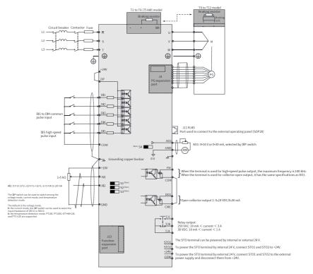
Figure 7-1 Standard wiring
