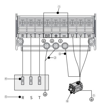
Figure 7-52 Main circuit grounding
