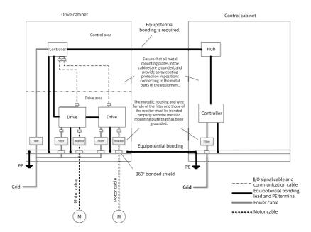
Figure 7-54 Recommended wiring for the cabinet system
