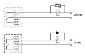
Figure 7-39 Anti-interference treatment for relay output terminals
