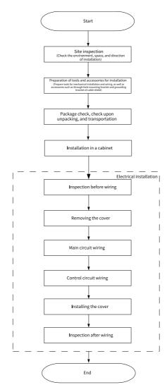
Figure 1-2 General installation process (T10 to T12 models)
