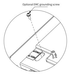
Figure 7-27 Disconnecting the optional EMC grounding screw
