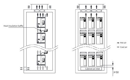
Figure 4-3 Position of the cabinet air inlet
