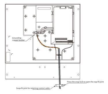
Figure 7-33 Grounding the shield of analog input cable
