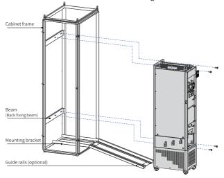
Figure 5-12 Fastening the AC drive to the fixing beams
