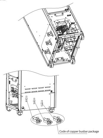
The following figures shows the installed copper busbar.
