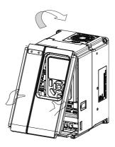
b. Align the cover, and then press the lower edge in the arrow direction.
