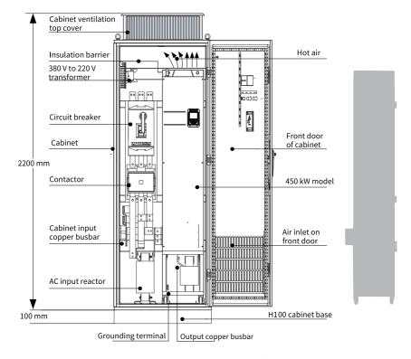
Figure 5-4 Recommended cabinet layout for T12 models
