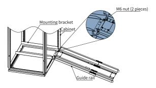
Figure 5-9 Mounting the guide rails on the cabinet
