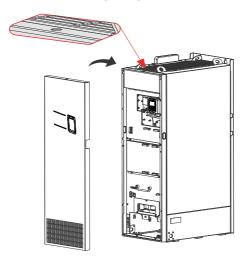
2. Drive six fixing screws into the holes with a screwdriver to fasten the cover.
