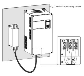
Figure 8-1 Installing an EMC filter
