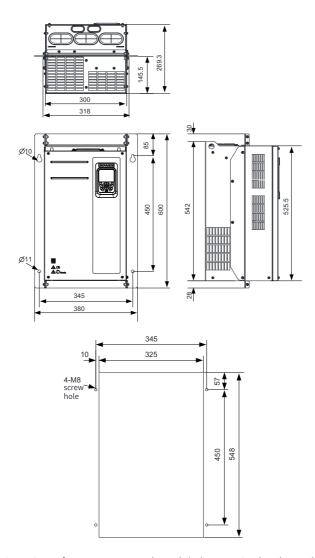
Figure 1-15 Dimensions of MD500-AZJ-A1T7 through-hole mounting bracket and holes (mm)
