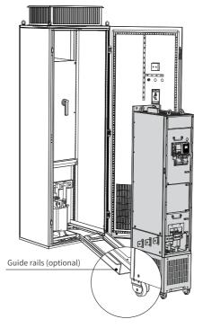
Figure 5-10 Aligning the casters with the guide rails
