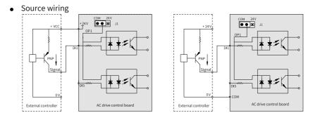
Source wiring where the 24 V power supply of the AC drive is used
