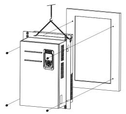
The following figure shows an AC drive that is through-hole mounted.
