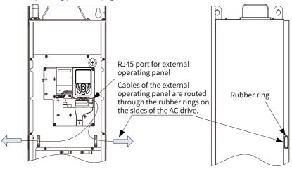
Figure 7-41 Wiring for connecting an external operating panel
