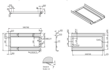
Figure 1-20 Dimensions of bottom mounting bracket for T12 models
