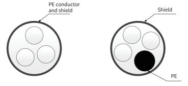
Figure 7-25 Recommended power cable types
