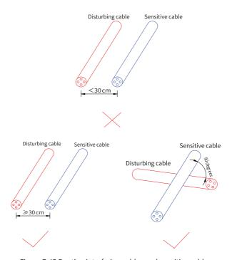
Figure 7-45 Routing interfering cables and sensitive cables
