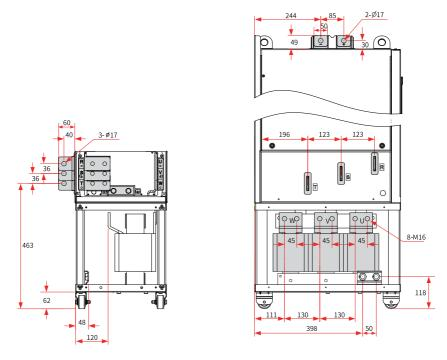
Figure 7-23 Main circuit terminal dimensions of T12 models (with output reactors) (mm)
