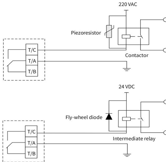
Figure 3-13 Anti-interference processing of relay output terminals
