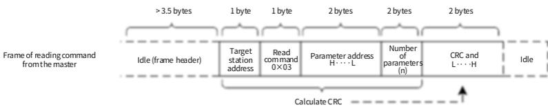
The host controller can theoretically read multiple continuous parameters at a time (i.e. N is up to 12). Do not stride the last parameter in this parameter group, otherwise the response error will occur.
