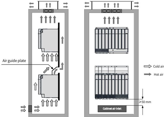
Figure 2-5 Position of the cabinet air inlet
