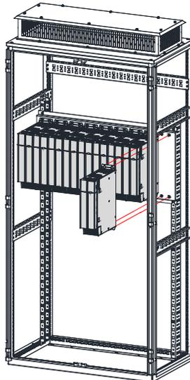
Step 4: Install the EMC grounding aluminum bar.
