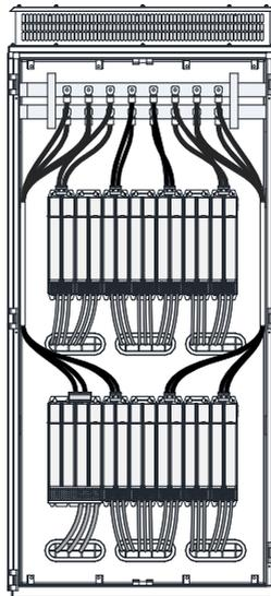
Step 8: Connect the control cable and PE grounding cable by referring to ["3 Electrical Installation"](#).
