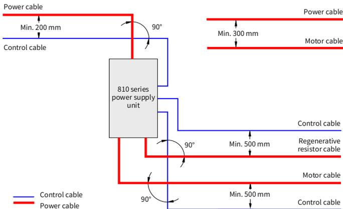
Figure 3-10 Cabling diagram
