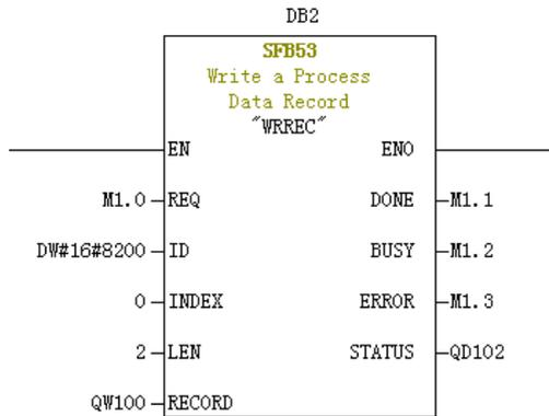
Note that before running an organization block, you need to download data blocks (above the function block with DB1 and DB2 used as examples) to the PLC. Otherwise, the DB block unloading error will be generated.
