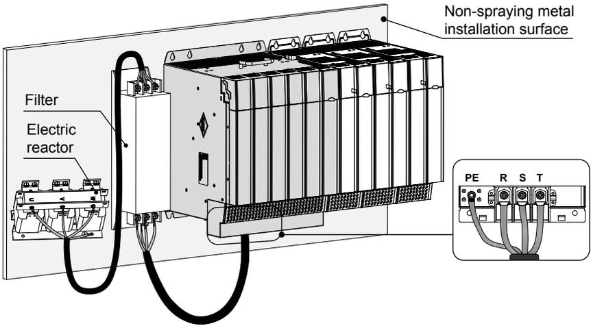
Figure 3-3 Protective grounding connection of main circuit terminals
