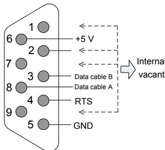
Figure 6-10 DB9 interface pins
