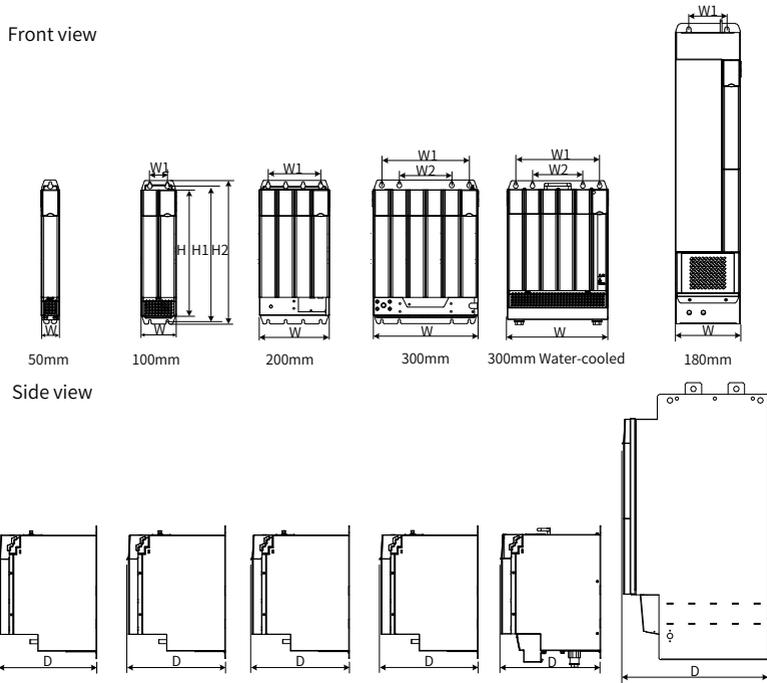
Figure 9-1 Overall dimensions of the power supply unit
