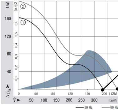
Fan maximum air flow Q<sub>max</sub>
