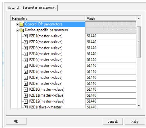
PZDx(master->slave) indicates the address used by the master station to write the slave station, and PZDx(slave->master) indicates the address used by the master station to read the slave station. PZD1 to PZD12 displayed in decimal are available. To set PZD3(master->slave) to F0-12, enter 61452.
