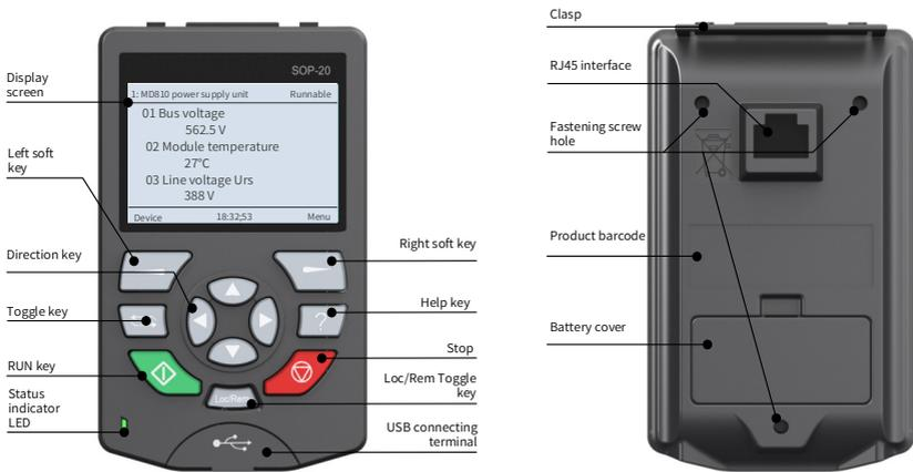
Figure 4-5 Appearance of external LCD operating panel
