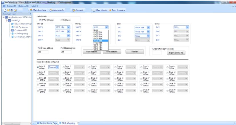
2) Mapping relation between PLC I/Q addresses and process data
