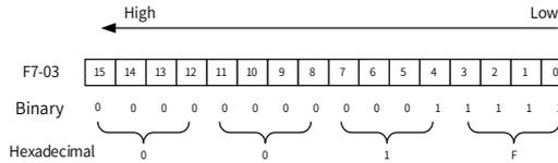
The method of viewing other state parameters is the same as F7-03 (Running display parameter 1). The corresponding relation between the state parameters and every byte of F7-03 (Running display parameter 1), F7-04 (Running display parameter 2), and F7-05 (Stop display parameter) is as follows:
