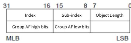
According to the preceding relation between the parameters and the object dictionary, when a parameter needs to be mapped to a PDO, you need only to write into group AF an object dictionary index and sub-index and data length corresponding to a parameter according to the preceding rules.
