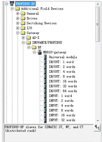
Step 3: Configure the actual hardware system, as shown in the following figure.
