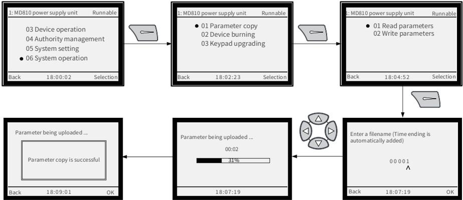
Figure 4-10 Parameter uploading
