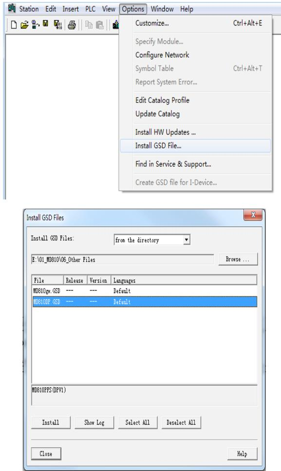
Click Install. After installation is complete, the PROFIBUS-DP module of MD810DP is displayed, as shown in the following figure.
