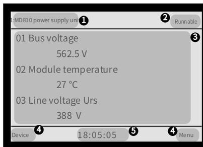
Figure 4-6 Main interface of the external LCD operating panel
