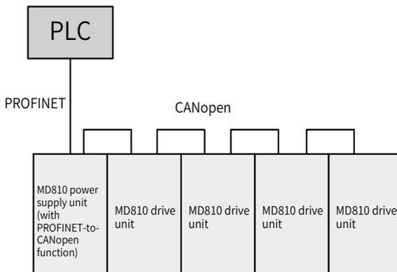
The network bridge function implements data exchange for a total of 30 nodes (including the power supply unit). Detailed data is as follows.
