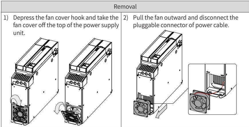
■ Installing the fan (80 mm x 80 mm) of a unit with equal height
