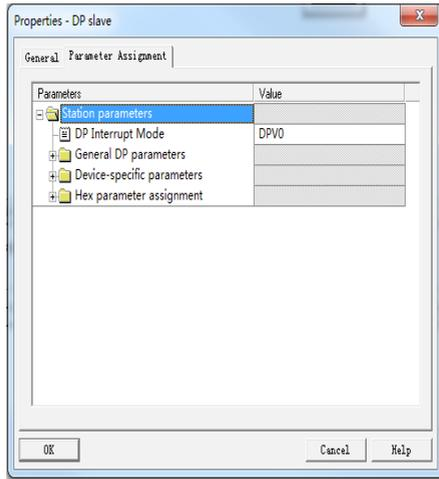
Parameters PZD1 to PZD12 are for customized periodic data exchange. They can be configured in hardware configuration. Double-click the MD810DP sign in HW Config, click "Device-specific parameters", and configure corresponding parameter addresses as required.
