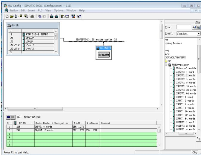
You can see various units with "IN/OUT", "INPUT" and "OUTPUT" on the right. They indicate IN and OUT data containing several words in these units.
