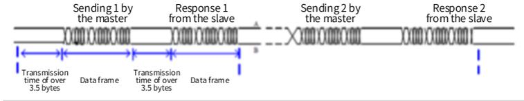
The built-in communication protocol of the 810 series power supply unit is the Modbus-RTU slave communication protocol. It enables the power supply unit to respond to an "inquiry/command" of the host or perform corresponding action and communication data response according to an "inquiry/command" of the host.
